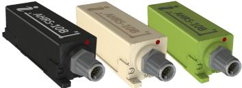
The Inertial Labs AHRS-10 utilizes 3-axes each of precision accelerometers, magnetometers and gyroscopes to provide accurate Heading, Pitch and Roll of the device under measure. Integration of gyroscopes' output provides high frequency, real-time measurement of the device rotation about all three rotational axes.
