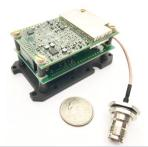
The Inertial Labs **INS-B-OEM** utilizes advanced single antenna GNSS receiver, barometer, 3-axes each of calibrated in full operational temperature range Advanced MEMS Accelerometers and Gyroscopes to provide accurate Position, Velocity, Heading, Pitch and Roll of the device under measure. **INS-B-OEM** contains Inertial Labs new on-board sensors fusion filter, state of the art navigation and guidance algorithms and calibration software.
