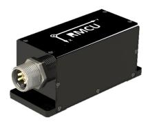
The Inertial Labs **RMCU** utilizes 3-axes each of precision MEMS accelerometers, miniature Fluxgate magnetometers and MEMS gyroscopes to provide accurate Heading, Pitch and Roll of the device under measure. Integration of gyroscopes' output provides high frequency, real-time measurement of the device rotation about all three rotational axes.
